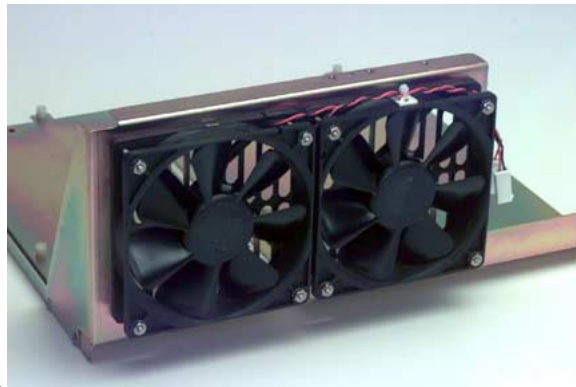
Fans on motherboard tray showing cable tie, nuts
