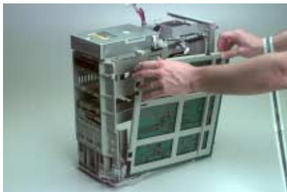
*Remove motherboard by tilting out from the top*
