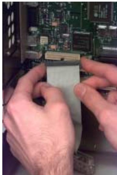
*Connect the AV module to the motherboard*
