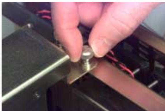
*Tighten nPOWER card screws*
