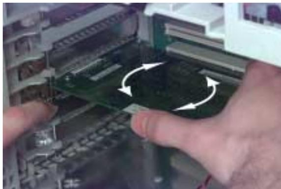
*Remove installed PCI card(s)*
