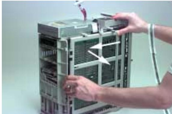
*Lift the latching tab and slide the motherboard forward*
