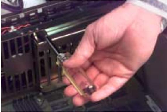
*Tighten securing nuts*
