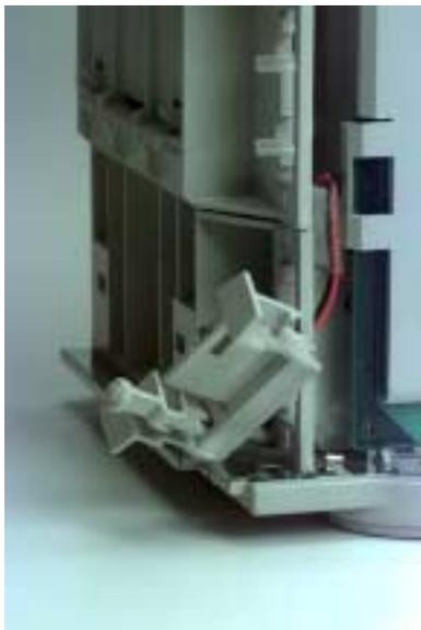
*Provide slack for removal of motherboard*
