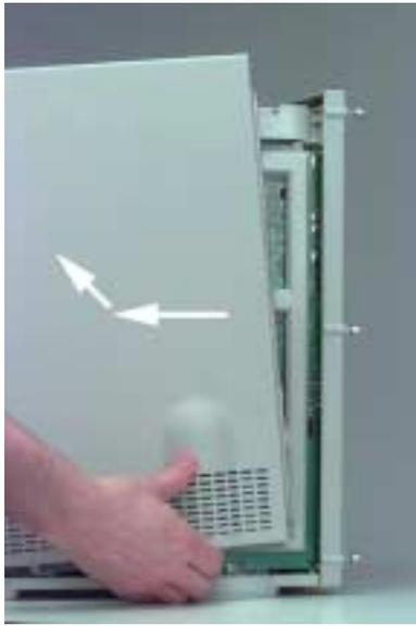
*Spread the sides slightly and remove the cover*
