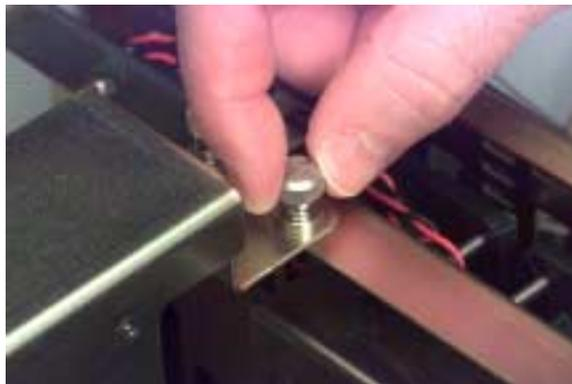
*Tighten nPOWER card screws*
