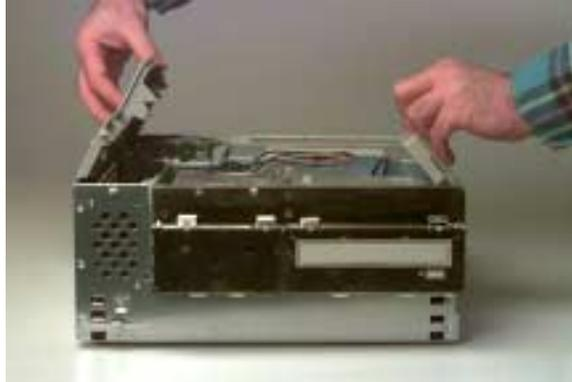
*Open the PCI card support cover and drive bay/power supply support stand*
